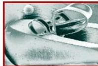
Coring of the silicone septum
