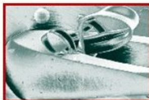
Coring of the silicone septum
